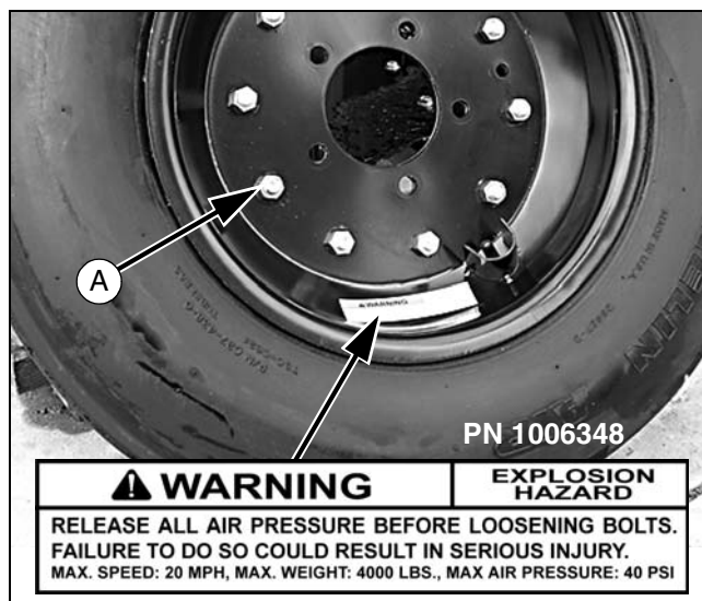
Figure 23. Split Rim Tire Servicing
